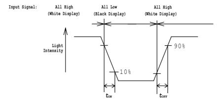
$t_{\mathrm{ON}}$ : Turn on time is the time for a photo detector output waveform to go from maximum value to 10% of its maximum.
